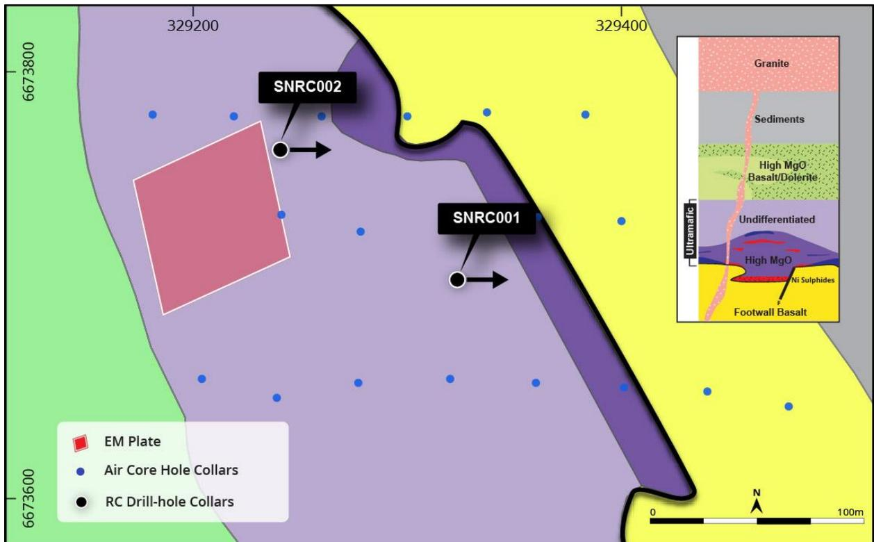
Figure 2 – Zoom of the T2 channel target area showing the location of the completed RC drill-hole collars and projection of the modelled DHEM conductor (plate) in relation to the interpreted geology
