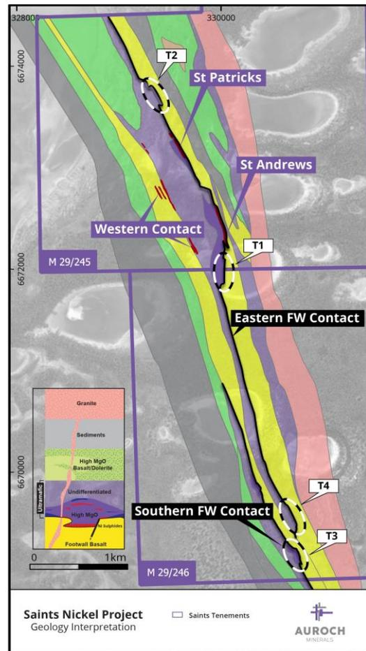
Interpreted geology map of the Saints Nickel Project highlighting the numerous channel targets in relation to the known nickel sulphide mineralisation (dark red) and ultramafic units (purple).
