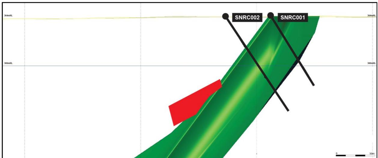
Figure 3 – 3D Cross-section at 6673720mN  $\pm$  60m through the T2 channel target area showing the location of the strong DHEM conductor (red plate) and completed RC drill-holes in relation to the modelled basal Eastern Footwall Contact (green). View is looking to the north
