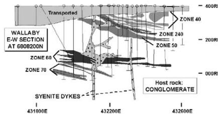
Wallaby E-W section. Stacked gold lodes are hosted by an actinolite-magnetite alteration pip (Coggon 2003)
