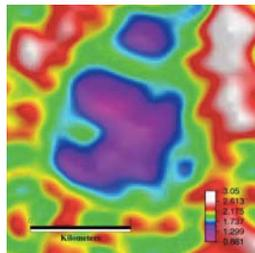
Resistivity - Conductive clay alteration and sulphide veins. A resistive silica cap can sometimes be detected.
