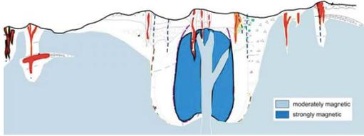
Genetic model of a porphyry, showing zones detectable by the magnetic method (top) and zones detectable by induced polarisation (chargeability/resistivity - bottom).
