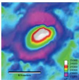
Magnetics - highly magnetic (magnetite-rich) core associated with mineralisation, coupled with a magnetically quiet (magnetite-destructive) alteration halo.(Above)
