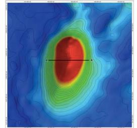
Wallaby deposit magnetic image. A "bullseye" magnetic anomaly is produced by magnetite accumulation.
