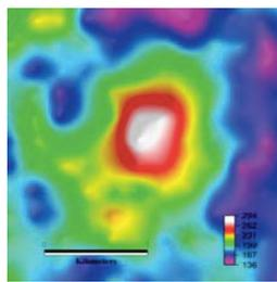
Radiometrics (K) - Radiometric response due to potassic alteration
