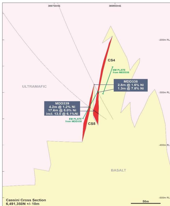
Figure 4: Cassini cross-section 6491350N with DHEM plates
