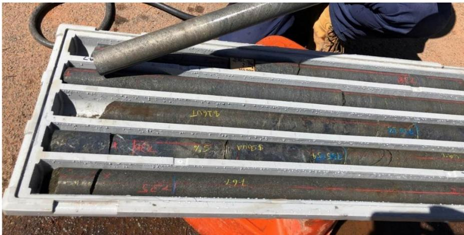
Figure 1: MDD339 core photo showing a section of heavy matrix nickel sulphides
